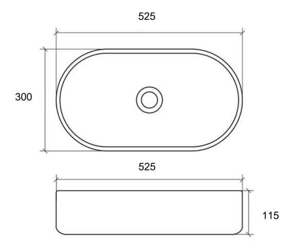
Dimensions are provided in millimeters and may vary slightly due to standard manufacturing processes
